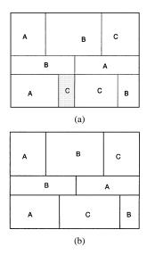
Fig. 1. Comparison between (a) C4.5 and (b) HIDER in the case of nonnested regions. C4.5 needs to split the space more times.
